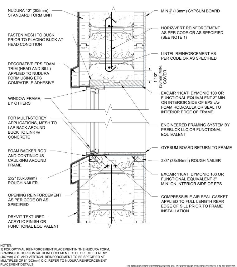
2) AIR BARRIER/DRAINAGE FLASHINGS TO BE INSTALLED AROUND COMPLETE OPENING PERIMETER AS PER TREMCO/NUDURA APPLICATION INSTRUCTIONS OR AS DETAILED BY LOCAL APPLICABLE CODES (CODE GOVERNS)
